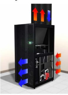
The InRow SC has a nominal net cooling capacity of 5kW and is primarily intended to serve the wiring closet and computer room spaces. Small data center users, possessing a ceiling plenum suitable for the unit heat rejection requirements and have no access to chilled water will often find the SC a compelling value given its scalability and easy of installation.
