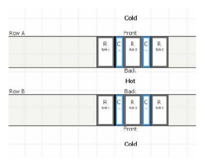
Figure 3 – InRow SC units and racks in multiple rows
